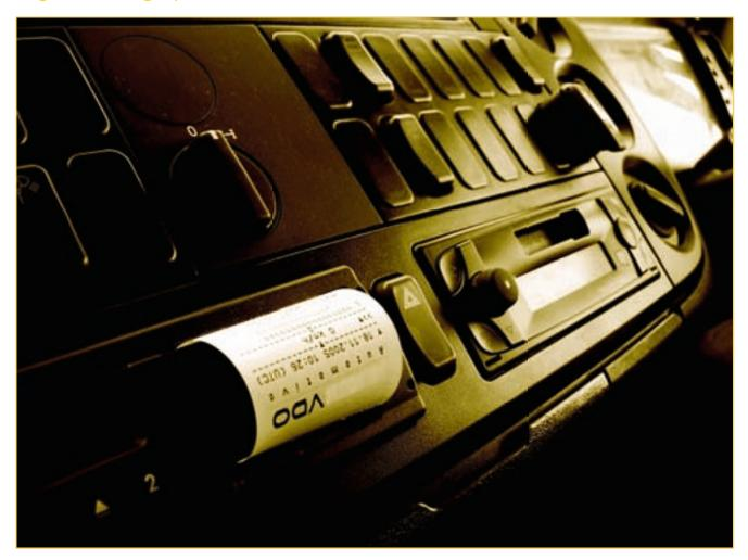
Digital tachographs work by storing digital data on the driver and vehicle in their own memory and separately on a driver's smart card. Transport undertakings must periodically download this data from the digital tachograph (known as the Vehicle Unit or VU) and from driver cards, and analyse the information to ensure that the rules have been complied with.
